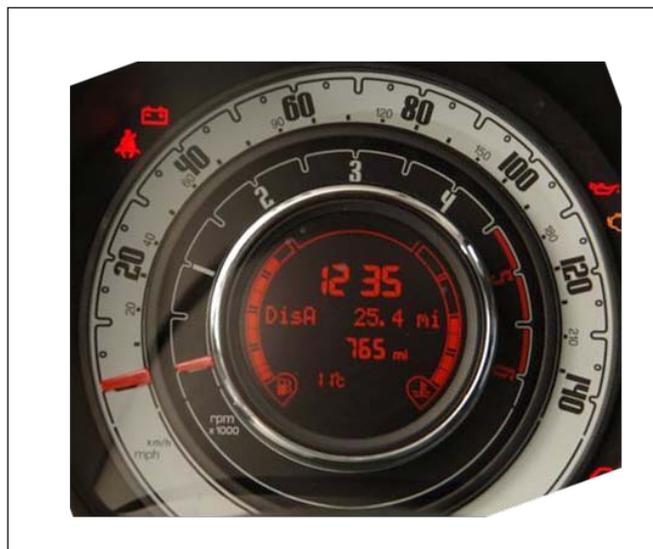
The speedometer is assembled with two dials on top of each other. The outer dial has two axes—mph and km/h. The inner dial is the rpm meter, which has a different scale and style. Another uncommon feature is that the body parts of both dials are hidden underneath; only the top needle parts are displayed. In the center of the gauge is an LED screen showing journey information. Using all these unique appearances, Highcharts provides enough flexibility to assemble a chart that looks very similar.
