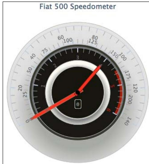
First we widen the needle by setting the `baseWidth` option to 7 pixels across and 3 pixels at the end of the needle. Then instead of having the needle narrowing down gradually to the end of the tip, we set the `baseLength` option to '90%' which is the position on the dial where the needle starts to narrow down to a point.
