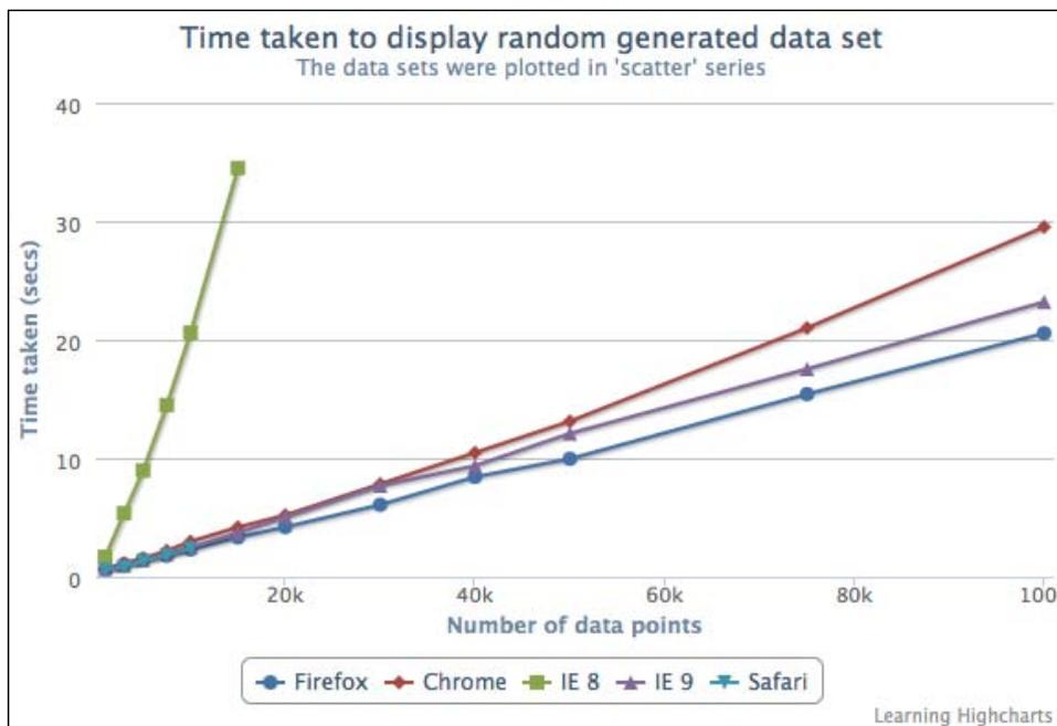
The most obvious part from the previous graph is the skewed line from IE8 performance. As IE8 uses the obsolete VML, it is around 2.5 times slower than IE9 at 1,000 data points, and approximately just under 10 times slower at 15,000 data points. Besides, it is difficult to time IE8 reliably after that point, as the long timing process has on-going interruptions by warning dialogs.
