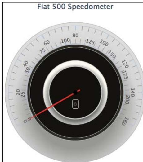
However, there is an issue arising in which the scale at the top axis has been disturbed; it is no longer between 0 and 140. This is because the default action for having a secondary axis is to align the intervals between multiple axes. To resolve this issue, we must set the `chart.alignTicks` option to `false`. After that, the issue is resolved and both axes are laid out as expected, as follows:
